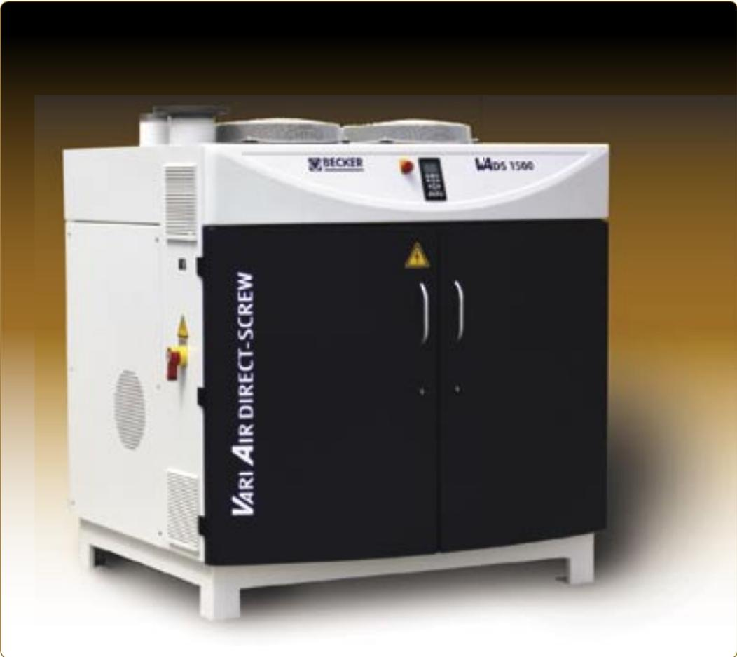
The VADS continually monitors the vacuum level in the process, and as leakage increases, the VariAir unit increases the speed of the pump, which increases the flow it produces. This results in maintaining a *constant holding pressure* on the product.
